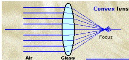
As the wave of propagation is still continuous, this slowing down bends the light beam, when it enters the new medium. It is similar to a bicycle changing direction when it enters sand from road. This basic principle is used in the construction of a lens.
