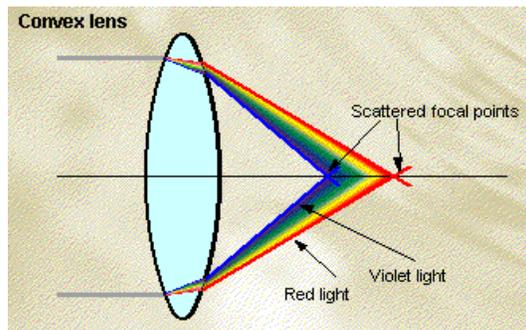
What is chromatic aberration? Simply it is this: Visible light is made of different colors and each color has a different frequency. These colors will bend differently compared to each other when they pass through a single convex lens, resulting in a scattered focal point (as shown in the diagram), meaning the picture will not be focused
