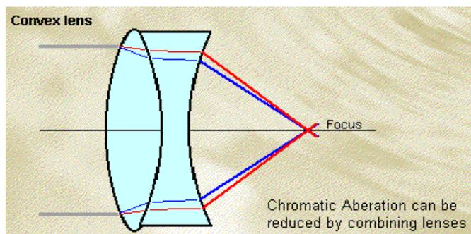
available which do not resolve the chromatic error accurately and are not compatible for use with color cameras, as they will not give a sharp focus for all the colors in the picture. The same reasoning and logic is applicable for the infra red frequency range also. For this
