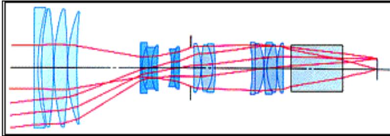
position shifts, the lens must be refocused. If two lenses are combined, it is possible to change the magnification without disturbing the focus. A
