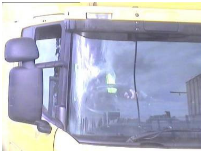
Example of a poor driver image taken using a CCTV camera without a polarizing filter to reduce the problem of windscreen reflection.
