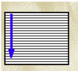
Vertical Resolution is limited by the number of horizontal scanning lines. In PAL it is 625 lines and in NTSC it is 525 lines. Using the Kell or aspect ratio factor the maximum vertical resolution is .7 of the number of horizontal scanning lines. Using this the maximum vertical resolution is
