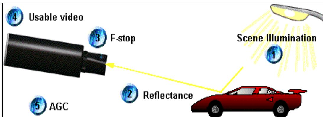
How does it work? Usually light falls on the subject. A certain percentage is absorbed and the balance is reflected and this moves toward the lens in the camera. Depending upon the iris opening of the camera a certain portion of the light falls on the CCD chip. This light then generates a charge, which is
